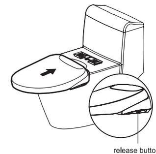
Slide the bidet seat all the way on to the catch plate. You will hear a click once the product is securely mounted to the catch plate.
