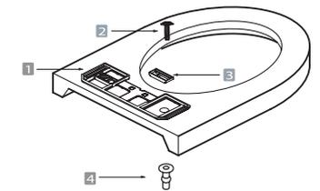
1 mounting plate 2 mounting screw 3 guide 4 rubber anchor
