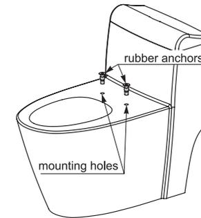
Remove the existing toilet seat and insert the rubber anchors into the mounting holes.
