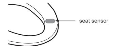
This appliance is equipped with a seat sensor and will not function unless it is occupied.
