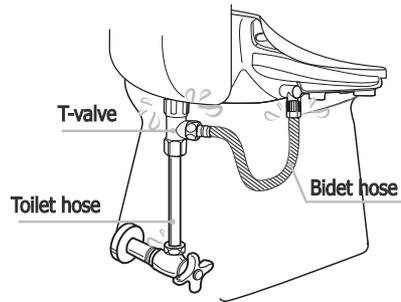
\*Do not overtighten connections.
