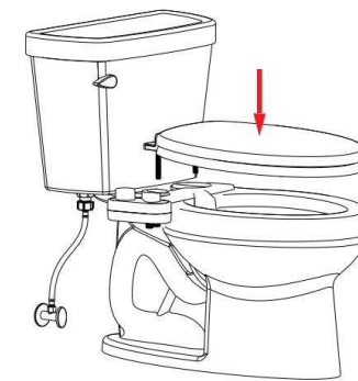
4. Install toilet seat
