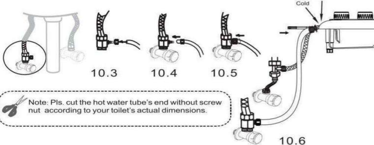
10.3: Unscrew the thumb nut from the hot water adapter
