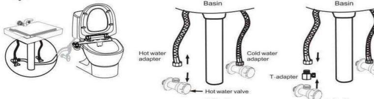
10.1: Pls. shut off the water supply valve first and then unscrew the basin's hot water adapter with your hands.
