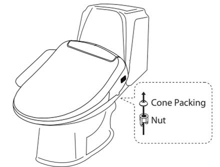
**7** Once the base plate is attached to the unit, align the unit and toilet fixture facing front, and then insert the mounting bolts to the toilet mounting holes.
