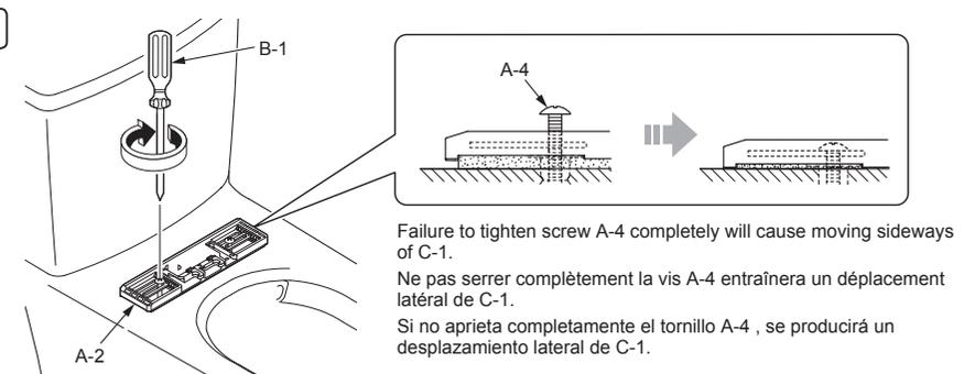
Failure to tighten screw A-4 completely will cause moving sideways of C-1.
